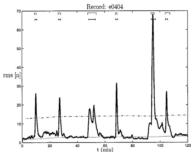
Fig. 4. Example of ST-T complex changes detection showing the annotated ( $\blacktriangle$ ) and detected ( $\text{---}$ ) episodes intervals. The baseline estimation,  $\xi[n]$ , (dotted line) and plus the  $\eta$  threshold (dash-dotted line) are plotted over the  $\text{rms}[n]$  series.
