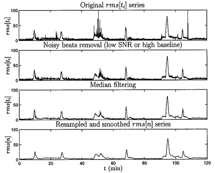
Fig. 2. Example of beats rejection (preprocessing stage) in the rms series of ST-T complex, and successive filtering stages (median filtering and exponential averaging). See text for details.
