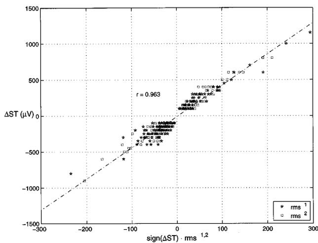
Fig. 7. Accuracy for estimating the ST segment deviation magnitude of the annotated events: regression line and correlation coefficient. See text for details.
