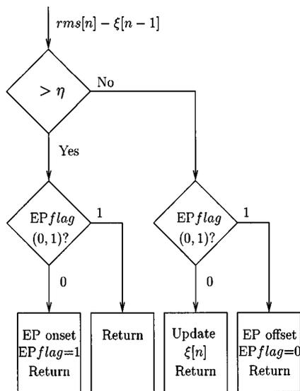
Fig. 3. Main structure of the detection algorithm that performs over the filtered  $\text{rms}[n]$  series.
